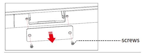
**Step 2** Insert the SDM-S into the port on the rear of the panel until firmly seated, using the 2 screws to secure it.
