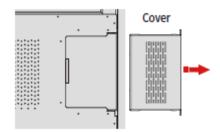
**Step 2** Push the OPS into the port on the rear of the panel until firmly seated, using the M4 screws to secure the OPS.
